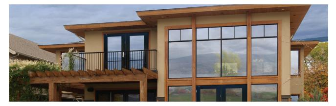
With high performance glazing it is possible, under certain conditions, to have condensation on the outside of the glazing. The glazing radiates to the sky and on a clear night that can reduce the temperature of the outside surface to below the dew point. Condensation will form similarly to the condensation on a car windshield and, once the sun comes up, the condensation will disappear.
