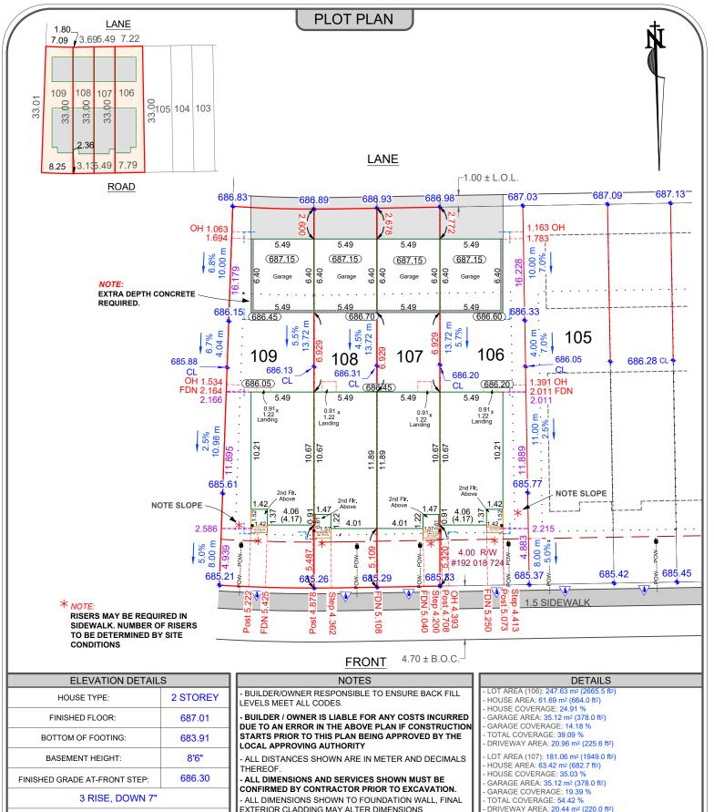
FINISHED GRADE AT-BACK OF HOUSE L-686.05, M-686.45, R-686.20 GRADE BELOW-BACK/SIDE DOOR SILL: GRADE BELOW-BASEMENT WINDOWS: WELL AS REQ'D TOP OF CONCRETE BASEMENT WALL 686.71 687 15 GARAGE FLOOR: SEE DETAIL SANITARY SEWER SERVICE INVERT: FOOTING SIZE: 0.20
